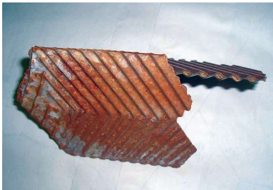
Figure 3 Scale buildup on one-year-old plate-and-frame heat exchanger
