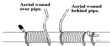
All four antennas of the WK1-E, WK2 and WK3 must be wrapped around the pipe.
